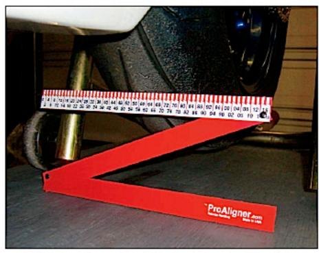
(Left) The ProAligner and the plastic sleeve it comes in. (Above) The ProAligner in position, resting against the leading edge of the rear wheel. (Bottom) A bike on a shop work table with the ProAligner in position and the instructions and a notepad in place near the front wheel. After sighting along the front and rear edges on each side of the front fire and comparing the readings on the ProAligner scale, a mechanic can calculate which way to move the chain adjusters to line up the wheels.
